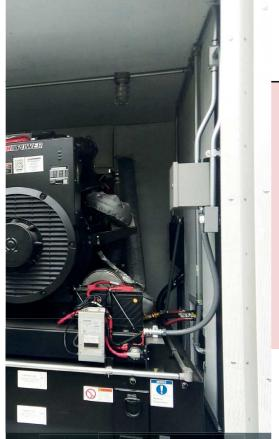
CK Power's hybrid battery charger uses a Girtz enclosure with a diesel engine from Volvo Penta or John Deere Power Systems.
